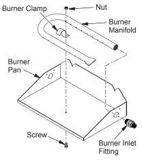
Figure 8 - Installing Burner
